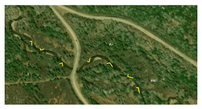
Figure 17: Lower sites on reach #1. Deflectors are most appropriate technique.
