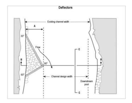
Figure 7: Conceptual drawing of a log framed deflector (source DFO 2008).
