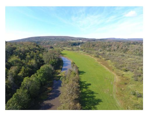
Figure 76: Erosion site at the lower extent of reach #3 of the lower section of the Mull River. Bank stabilization and tree planting are recommended here.
