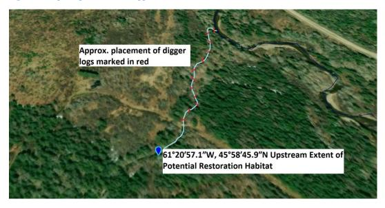
Figure 41: Satellite image showing approximate location and sequence of digger logs.
