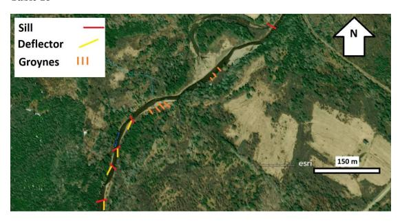
Figure 65: Approximate structure layout for reach #2 mid section Mull River.
