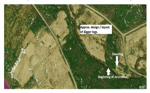
Figure 15: Red lines denote approximate location and design of digger log structures.
