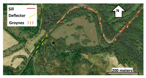
Figure 66: Approximate structure layout for reach #3 mid section Mull River.
