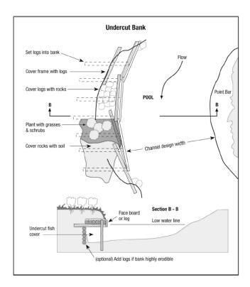
Figure 8: Diagram of an undercut bank structure
