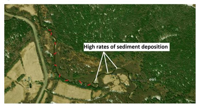
Figure 25: Red lines indicate approximate location of digger logs.
