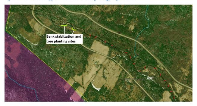
Figure 16: Approximate layout of instream restoration structures. Digger logs denoting in red.
