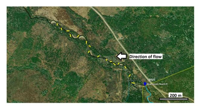
Figure 44: Approximate placement of deflector structures in upper section reach #2.
