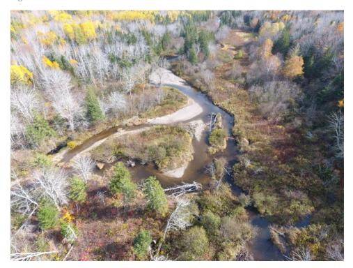
Figure 20: Aerial photo of debris complex and multi-thread channel development.
