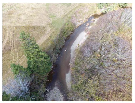
Figure 23: Bank erosion issues on the left. Restoration work should include tree planting and bank stabilization.
